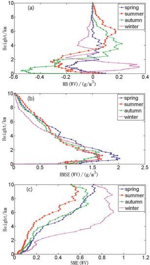
FIG. 4. Comparison results for the retrieved water vapor density profiles in the four seasons: (a) MB, (b) RMSE, and (c) NME.
