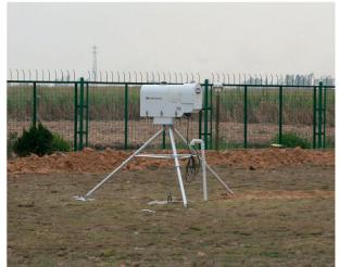
FIG. 2. The ground-based, 35-channel microwave radiometer.
