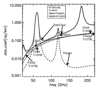
FIG. 1. Atmospheric absorption bands of microwave radiation between 20 and 220 GHz.
