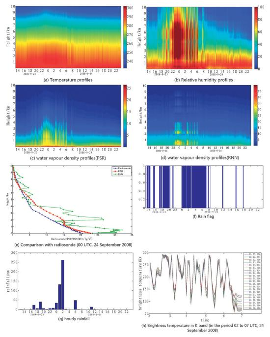
FIG. 10. Meteorological data at Nansha in the period 23–24 Sep 2008: (a) temperature profiles, (b) relative humidity profiles, (c) water vapor density profiles (PSR), (d) water vapor density profiles (RNN), (e) comparison with radiosonde (0000 UTC 24 Sep 2008), (f) rain detector data, (g) hourly rainfall, and (h) K-band brightness temperature.
