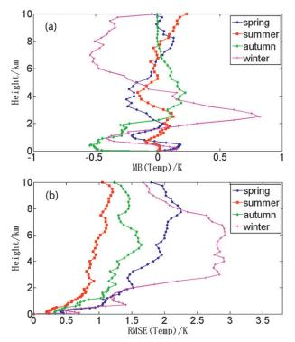
FIG. 3. Comparison results for the retrieved temperature profiles in the four seasons: (a) MB and (b) RMSE.
