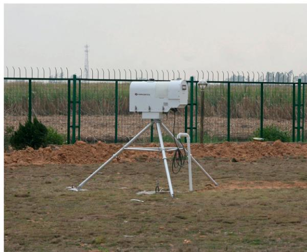
FIG. 2. The ground-based, 35-channel microwave radiometer.
